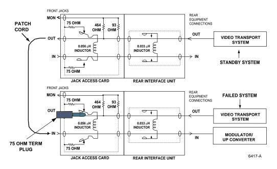
Figure 21. Bypass Failed Video Transport System
